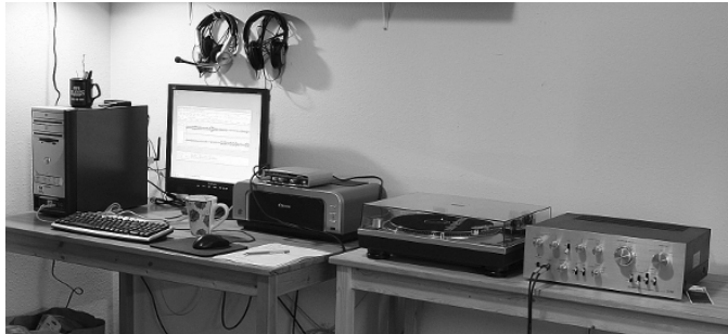
Figure 3-14: From the right to left: nice old Pioneer stereo amp, Audio Technica three-speed turntable, color printer, M-Audio MobilePre, screen, headsets, three-core CPU wedged into salvaged E-Machine case
