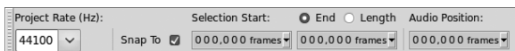
Figure 4-12: Setting the correct frame rate for CD audio in the Selection toolbar
