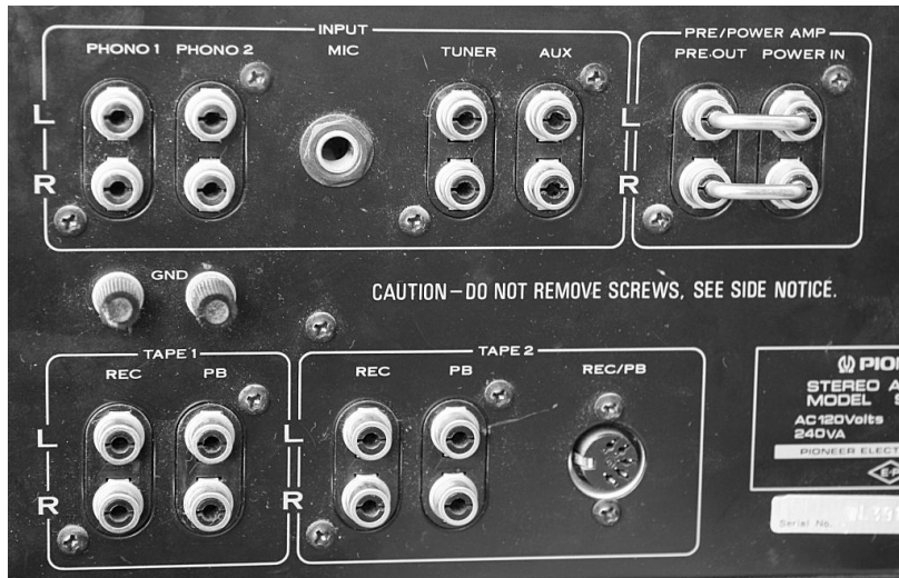
Figure 2-2: This is the back of a treasured old but versatile Pioneer stereo amplifier. It can connect two turntables (it even has proper ground connectors for turntables), two tape decks, a microphone, a tuner, another amp, a preamp, and an Aux connector for a CD player or other input devices.
