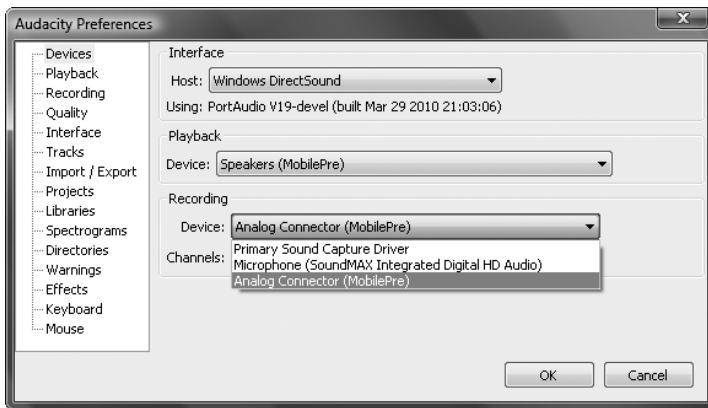
Figure 4-4: Setting the correct recording and playback devices in the Edit > Preferences > Devices dialog on Windows
