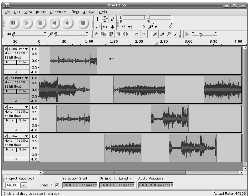
Figure 9-4: Clips can be moved independently all over the place with the Time Shift tool, even to different tracks.
