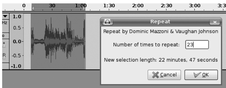
Figure 9-29: Creating a simple loop by using a short clip and selecting Effect > Repeat
