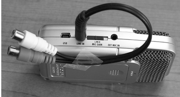
Figure 4-2: Zoom H2 with a two-RCA-to-1/8" stereo adapter for connecting to a mixing console
