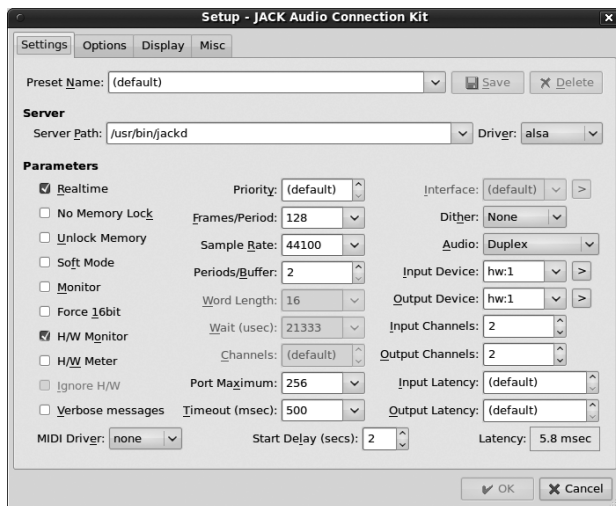
Figure 13-6: Selecting your audio devices and configuring JACK in the Qjackctl Setup dialog
