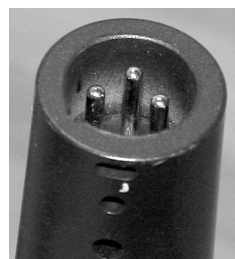
Figure 2-8: Behringer dynamic mic showing off its three-pin male XLR connector
