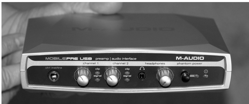
Figure 2-3: M-Audio MobilePre, front. From left to right: Channel 1 1/4" mono TRS jack, Ch. 1 and 2 gain controls, clip LEDs, headphone port, headphone volume knob, phantom power switch, phantom power LED, and power LED
