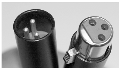
Figure 2-6: Here is a three-pin male XLR plug and a three-pin female XLR plug.
