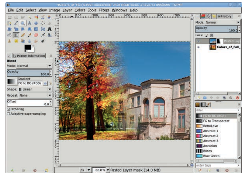
Blending two images together by applying a gradient to a layer mask
