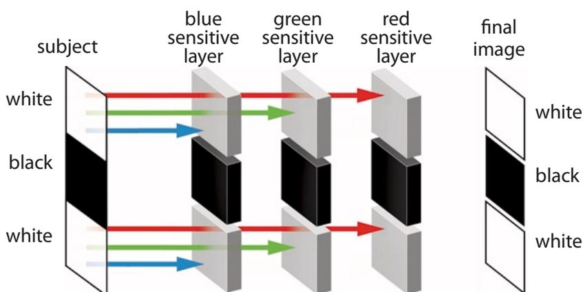
Figure 1.6: X3 sensor with no color interpretation errors
