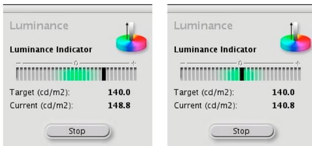
◀ *Figure 2-12: Set the luminance using your brightness control of the monitor to a target value of 120–150 cd/m<sup>2</sup>.*
