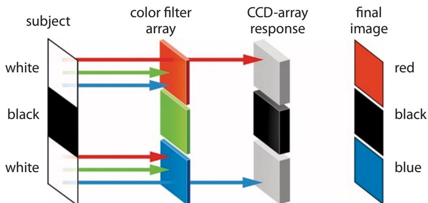
Figure 1.5: CCD / color mosaic sensor with color interpolation errors
