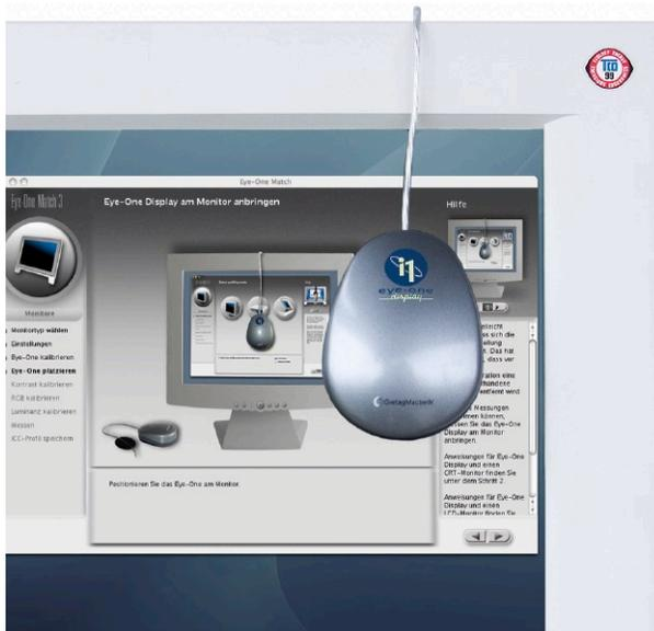
◀ *Figure 2-9: Eye-One Display colorimeter*
