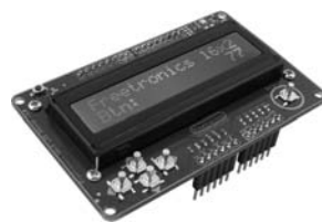
Figure 13-6: The Freetronics LCD & Keypad shield
