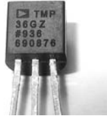
Figure 4-40: TMP36 temperature sensor
