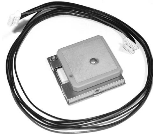
Figure 13-3: A long GPS-receiver-to-shield cable
