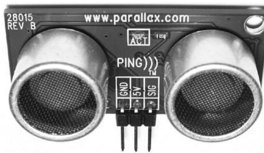
Figure 12-26: The Ping))) ultrasonic distance sensor
