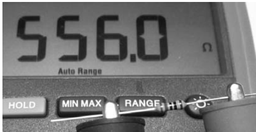
Figure 3-4: Multimeter measuring a 560-ohm 1 percent tolerance resistor
