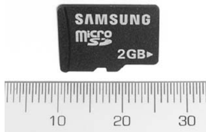
Figure 8-23: A microSD card with a 2GB capacity
