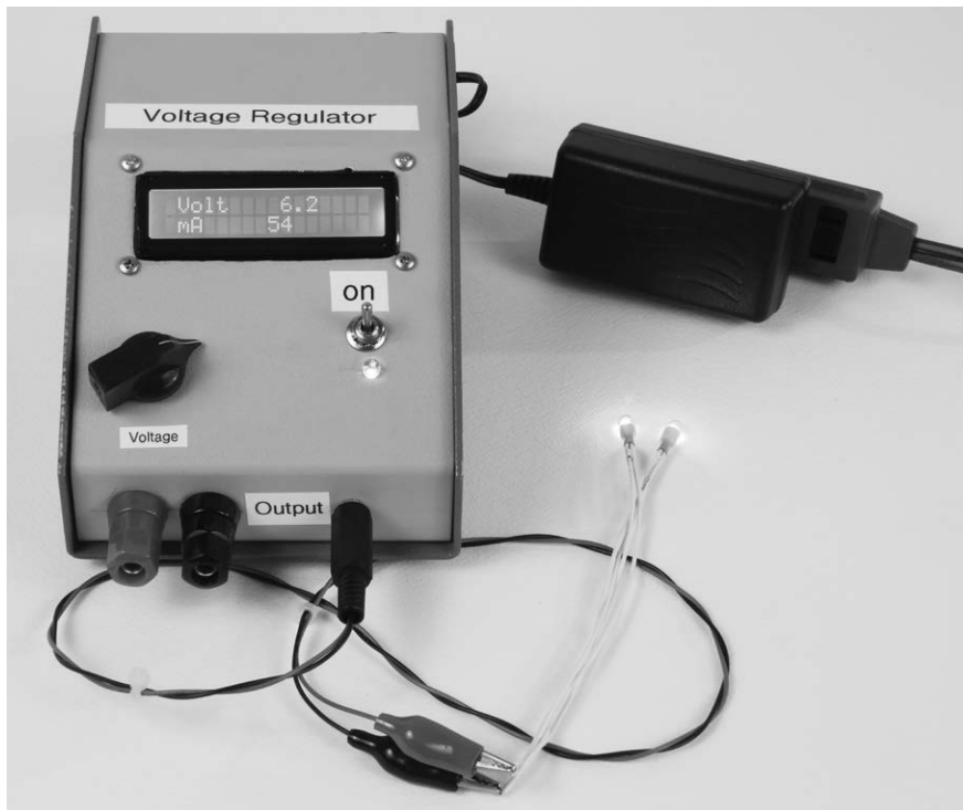
Figure 3-9: The completed Regulated Power Supply
