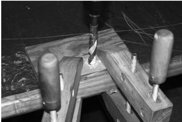
Figure 4-13: Drilling a large hole in the acrylic. Note that the acrylic piece is securely clamped down.
