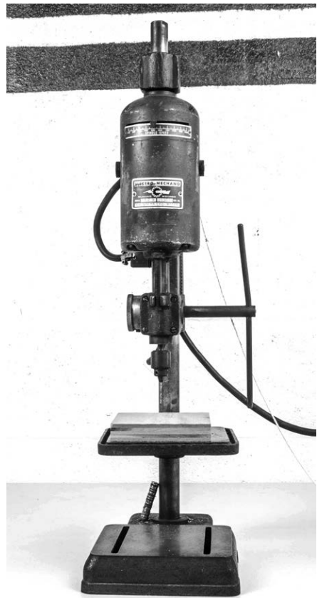
Figure 0-18: The small Electro-Mechano drill press I use for drilling PCBs
