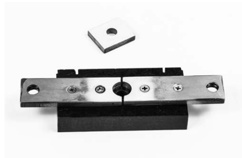
Figure 6-26: Battery Saver contacts after silver plating with Cool Amp
