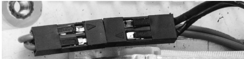
Figure 6-5: A pair of mating connectors used to connect the solenoid
