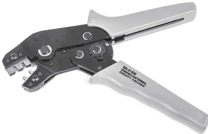
Figure 0-20: Crimping tool used to crimp 0.100 crimp connectors to 26-, 28-, and 30-gauge wire
