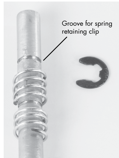
Figure 6-19: The upper section of the release bar. There are two grooves in the bar; the lower one was made in error. The springs used on the release rod were selected from a standard spring assortment from Ace Hardware and cut down to fit the project
