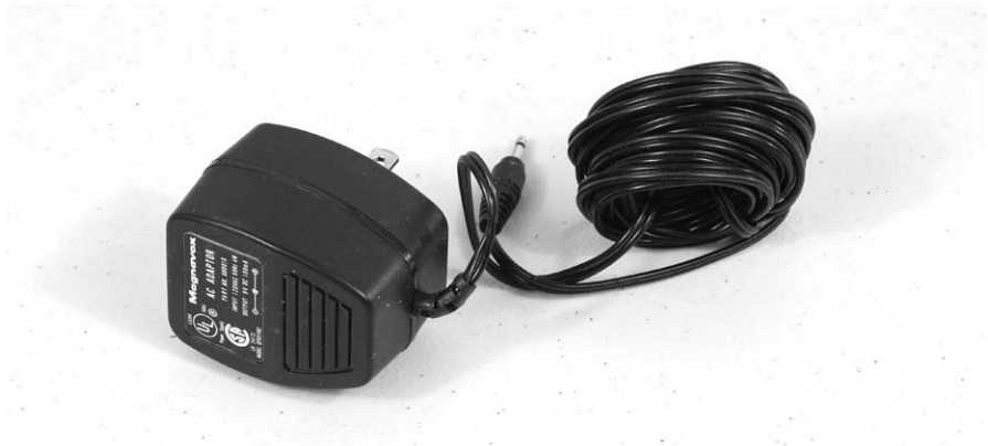
Figure 5-1: I used a Magnavox AC adapter, but any similar power supply with a DC output from 7.5V to 12V should work. These are readily available online and cost from under $1.00 to about $3.00.
