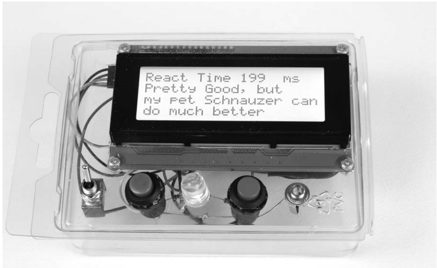
Figure 1-4: This was the Reaction-Time Machine’s original, primitive package, which worked but turned out to be too flimsy. The vinyl was only 0.018 inches thick.
