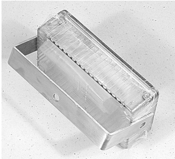
Figure 5-12: The enclosure for the basic Garage Sentry can be mounted with the bracket so it can be tilted or rotated to point the transducers in the correct direction.
