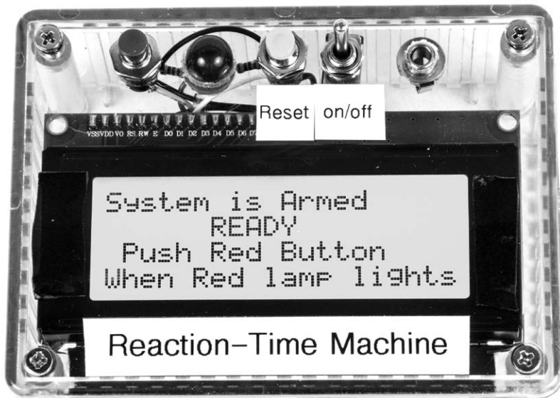
Figure 1-7: The completed Reaction-Time Machine mounted in the Hammond 1591 BTCL clear plastic enclosure
