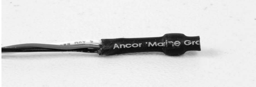
Figure 7-21: This LM35 temperature IC is completely encapsulated in a short length of heat-shrink tubing with a sealant thermal gel. The thermal gel can barely be seen where the wires enter the tubing.
