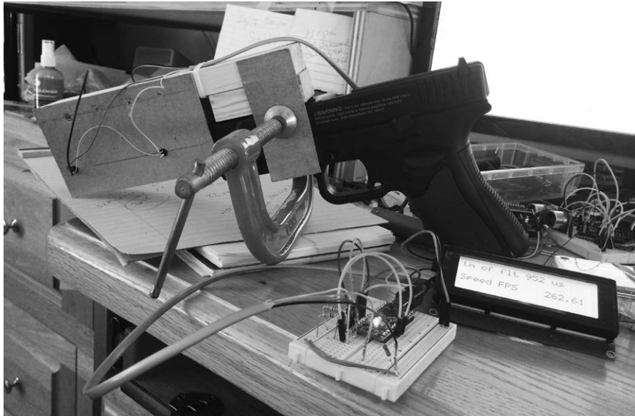
Figure 8-6: Photoelectric sensors in an early prototype, attached to a Crossman 0.177 caliber air pistol. The setup was obviously primitive, using a C-clamp to hold the channel to the weapon. Because the test channel was so simple, I set it up on my desk.
