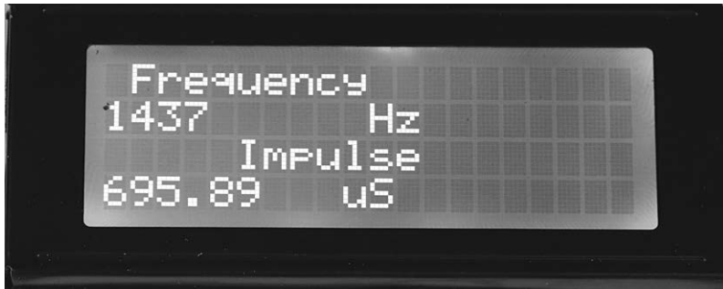
Figure 9-9: The display of the Square-Wave Generator, showing the frequency and the impulse time
