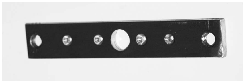
Figure 6-4: A copper bus bar, drilled out for the Battery Saver
