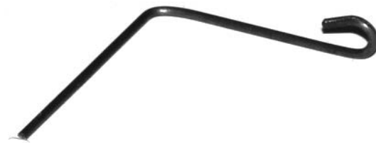
Figure 2-16: This is how the limit pins are formed. A good pair of needle-nose pliers does the trick.
