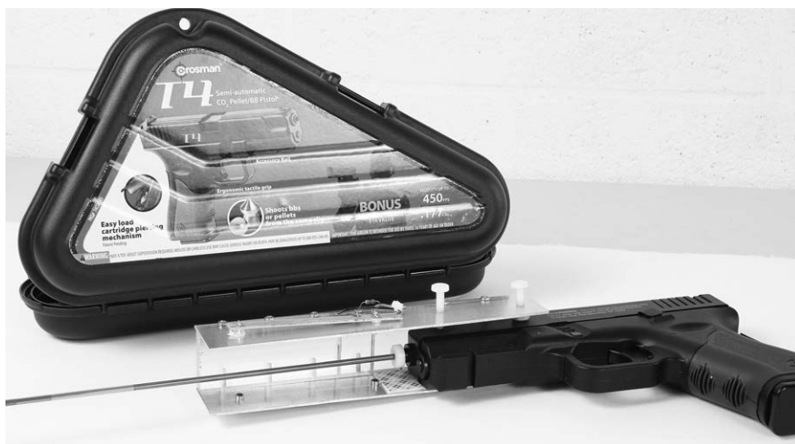
Figure 8-28: Using a small diameter brass rod with a Teflon end to set up proper alignment between the barrel of a Crossman T-4 CO 2 pistol and the sensor/detectors in the sensor channel
