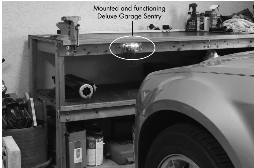
Figure 5-17: Completed Deluxe Garage Sentry mounted on my garage workbench with the car in place
