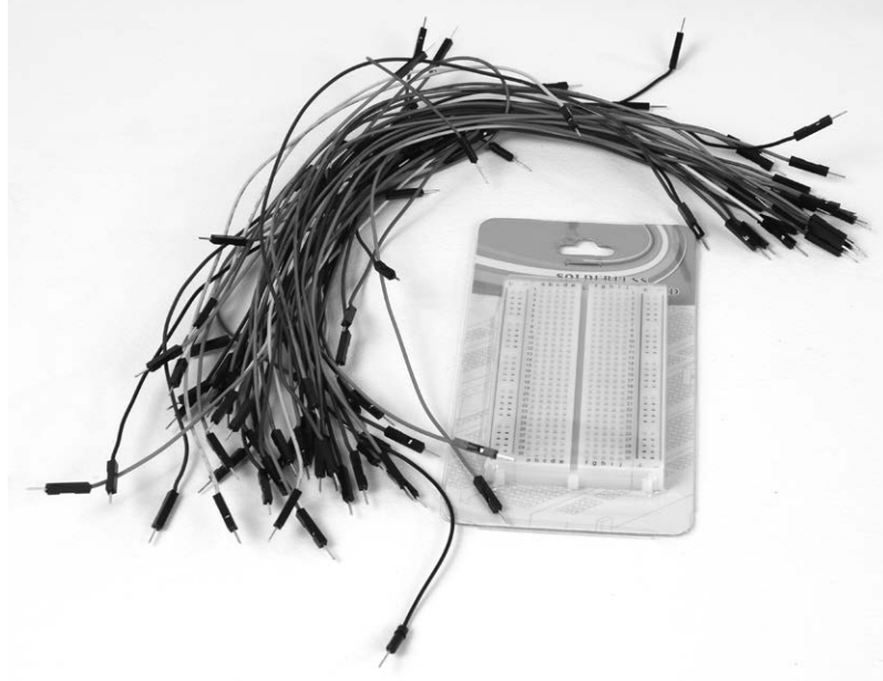
Figure 2-8: Typical small breadboard and plug-in wires
