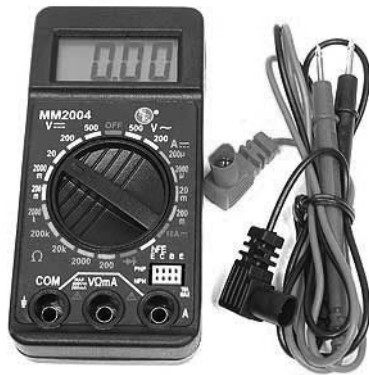
Figure 2-5: Multimeters are handy for many projects and useful to have around the house. They're available from a variety of sources at a range of prices. I use this cheap one from Electronic Goldmine, but if you plan to do high-voltage experiments, invest in a really good multimeter.
