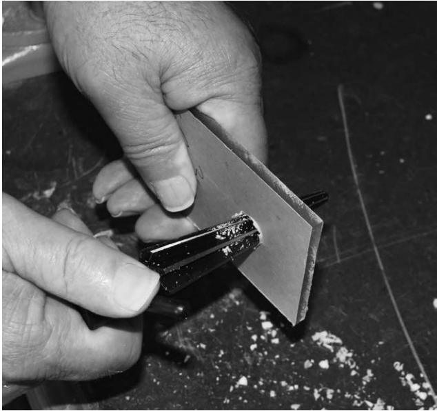
Figure 4-14: Using a tapered reamer to enlarge the bearing hole to the finished dimension
