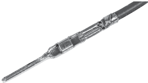
Figure 0-21: A male crimp connector properly crimped using the crimping tool
