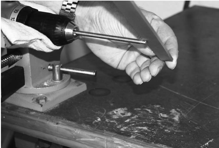
Figure 4-16: Reducing the diameter of the threaded shaft
