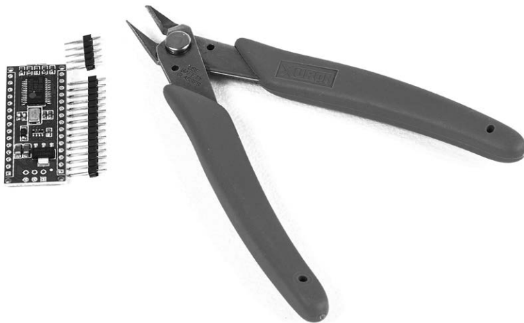
Figure 0-2: The Arduino Pro Mini clone, with the header pins trimmed to length. The 5-pin strip fits on the end of the board.
