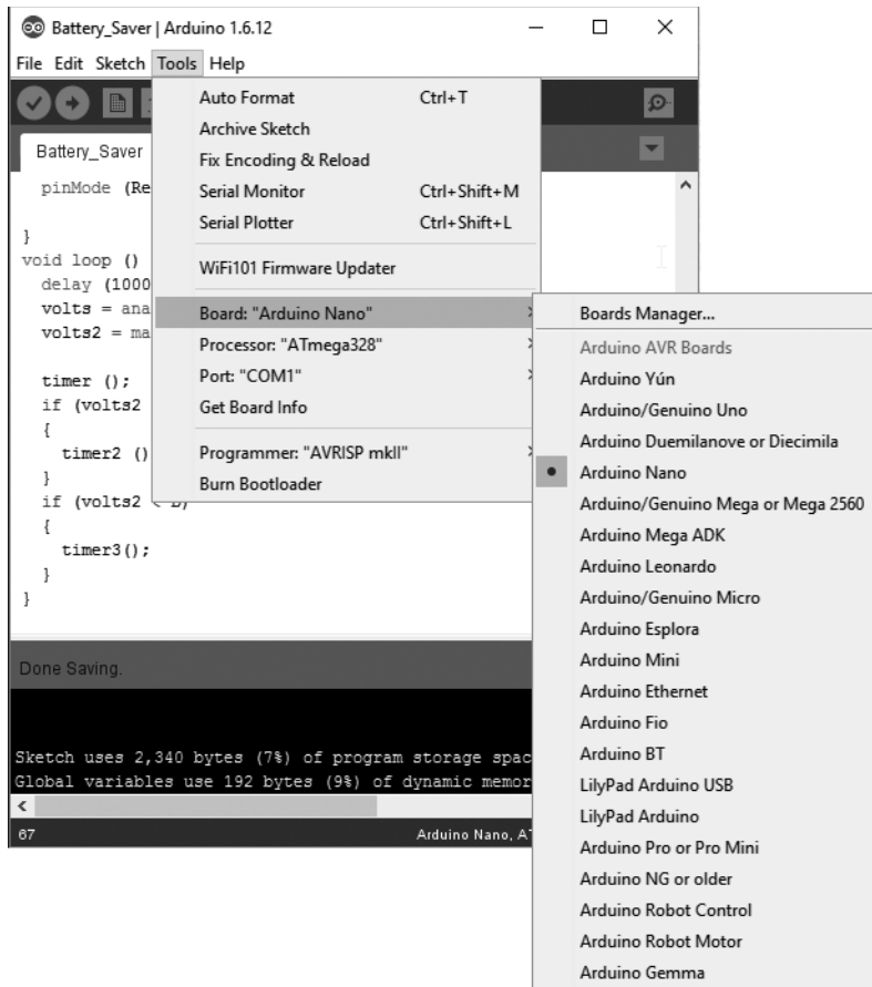
Figure 0-8: The sketch window, with the Tools menu open. I selected Arduino Nano with the ATmega328.
