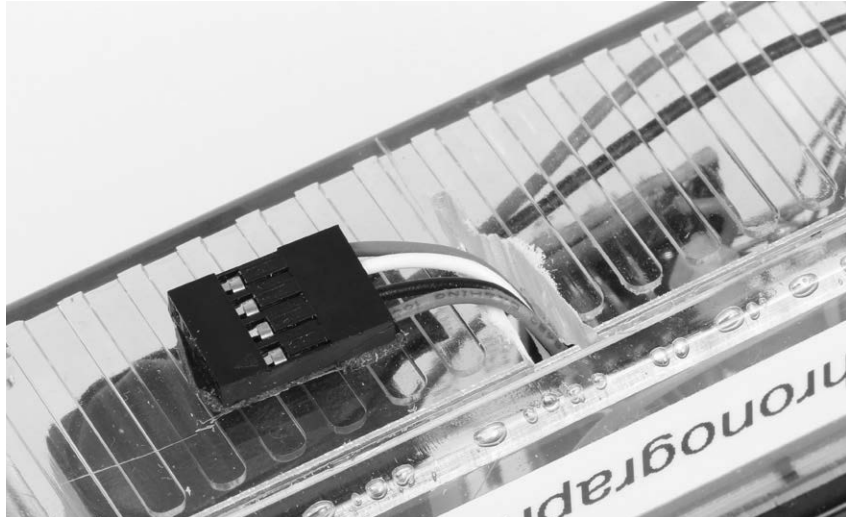
Figure 8-11: A slot in the enclosure for threading the four-pin sensor channel connector through. The connector is mounted with double-sided adhesive
