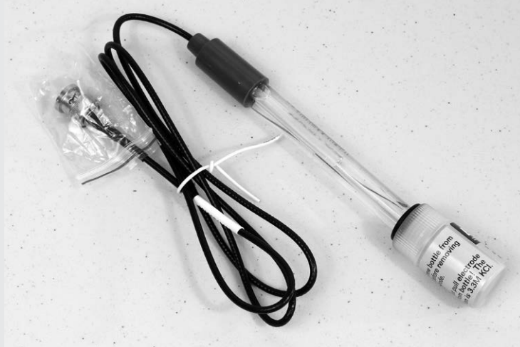
Figure 7-5: The pH probe I used for this project. The tip is protected in a small vial of KCl solution with a rubber seal.
