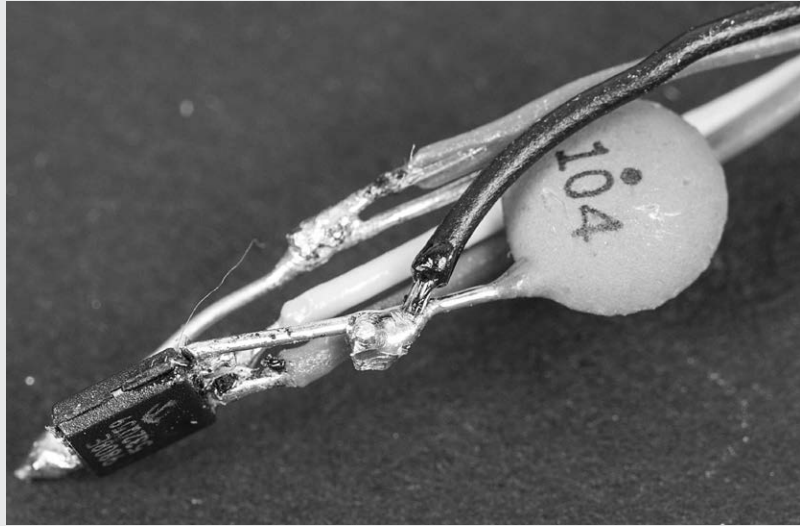
Figure 10-2: The MCP9808 with wires soldered directly
