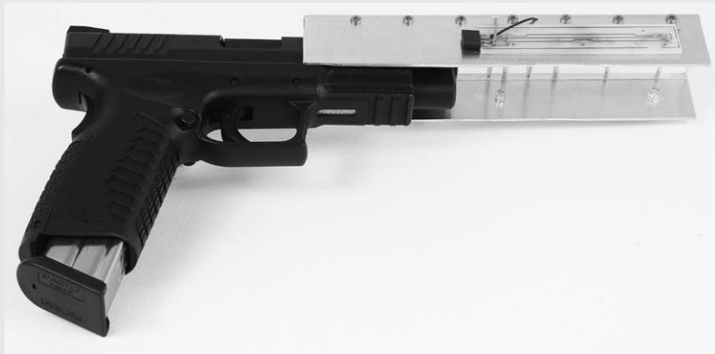
Figure 8-29: A Smithfield XP/M 9 mm pistol set up with the sensor channel for the Full Ballistic Chronograph. The magazine is intentionally inserted backward for safety reasons.
