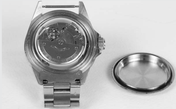
Figure 4-2: An automatic watch with the back removed, exposing the pendulum and the fulcrum (the screw in the center), which combine with a ratchet assembly to wind the watch's mainspring
