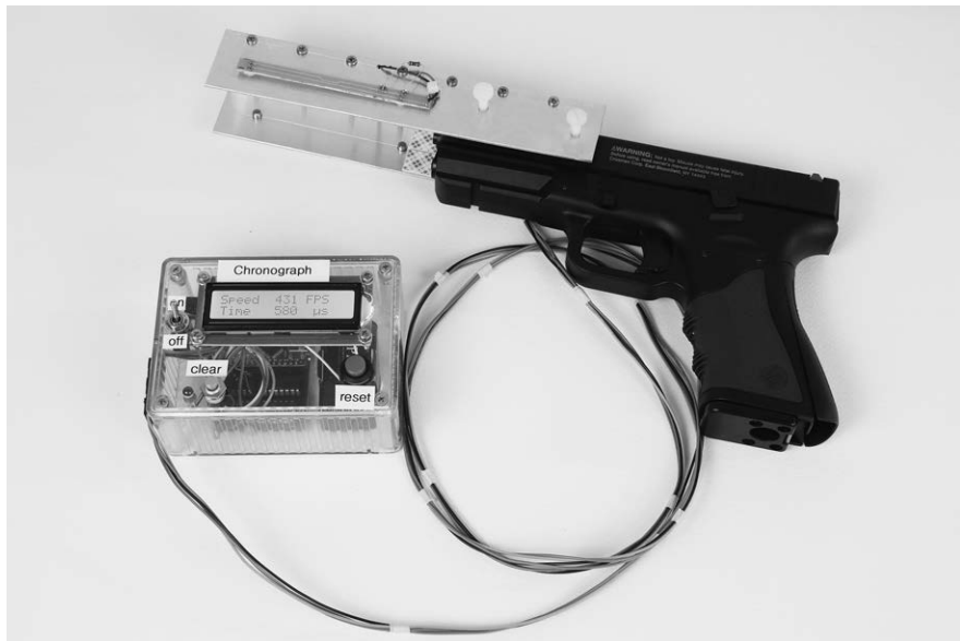
Figure 8-27: The completed Full Ballistic Chronograph with the acceleration channel mounted to a Crossman 0.177 caliber pellet gun
