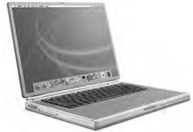
The PowerBook G4 was notable for its ultrathin titanium case.
