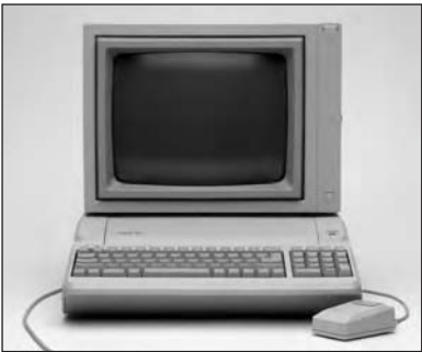
The Platinum Apple IIe, shown here with an optional mouse, featured a built-in numeric keypad and came standard with an extended 80-column card.
