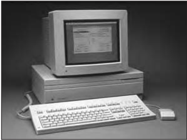
The Mac IIx used the same “Open Mac” case as the original Mac II, but came standard with dual 1.44MB 3.5-inch disk drives and was easier to upgrade.
