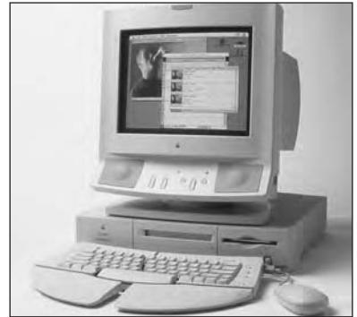
The Centris 660AV (shown here with an Apple Adjustable Keyboard) got its name from its audio/video card with RCA and S-video ports.
