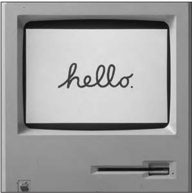
The original Macintosh had only 128K of memory, a 400K 3.5-inch disk drive, and a WYSIWYG monochrome monitor.
