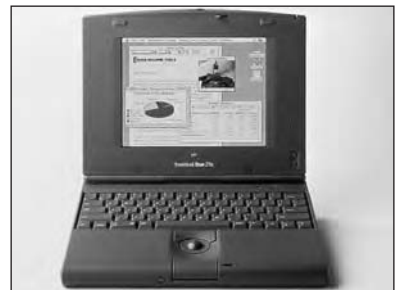
The PowerBook Duo 270c featured a 265-color, 640-by-480 pixel, active-matrix LCD.
