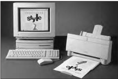
The Mac LC II (shown here with a StyleWriter) came in the same “pizza box” as the LC, but used a 16MHz 68030 instead of a 68020.
