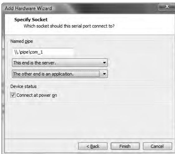
Figure B-2: Named pipe configuration
