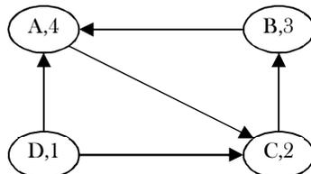
The last step is performing DFS on this reversed graph *G<sub>r</sub>*. While doing *DFS*, we need to consider the vertex which has the largest DFS number. So, first we start at *A* and with *DFS* we go to *C* and then *B*. At *B*, we cannot move further. This says that {*A, B, C*} is a strongly connected component. Now the only remaining element is *D* and we end our second *DFS* at *D*. So the connected components are: {*A, B, C*} and {*D*}.
