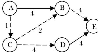
The final minimum cost tree which Dijkstra's algorithm generates is:
