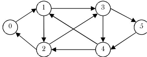
If we start at vertex 0, we can select the edge to vertex 1, then select the edge to vertex 2, then select the edge to vertex 0. There are now no remaining unchosen edges from vertex 0:
