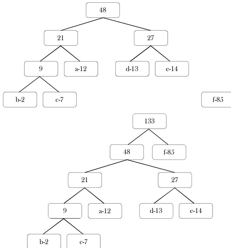
Once the tree is built, each leaf node corresponds to a letter with a code. To determine the code for a particular node, traverse from the root to the leaf node. For each move to the left, append a 0 to the code, and for each move to the right, append a 1. As a result, for the above generated tree, we get the following codes:
