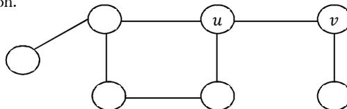
In the above graph, if we remove the edge  $uv$  then the graph splits into two components. For this graph,  $uv$  is a bridge. The discussion we had for cut vertices holds good for bridges also. The only change is, instead of printing the vertex, we give the edge. The main observation is that an edge  $(u, v)$  cannot be a bridge if it is part of a cycle. If  $(u, v)$  is not part of a cycle, then it is a bridge.
