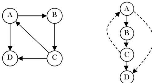
Now, as per the algorithm, performing *DFS* on this *G* graph gives the following diagram. The dotted line from *C* to *A* indicates a back edge. Now, performing post order traversal on this tree gives: *D, C, B* and *A*.
