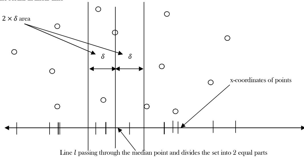
Let  $\delta = \min(L, R)$ , where  $L$  is the solution to first sub problem and  $R$  is the solution to second sub problem. The possible candidates for closest-pair, which are across the dividing line, are those which are less than  $\delta$  distance from the line. So we need only the points which are inside the  $2 \times \delta$  area across the dividing line as shown in the figure. Now, to check all points within distance  $\delta$  from the line, consider the following figure.
