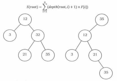
In the above expression, depth(root, i) + 1 indicates the number of comparisons for searching the  $i^{th}$  element. Since we are trying to create a binary search tree, the left subtree elements are less than root element and the right subtree elements are greater than root element. If we separate the left subtree time and right subtree time, then the above expression can be written as:
