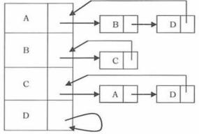
Since vertex A has an edge for B and D, we have added them in the adjacency list for A. The same is the case with other vertices as well.
