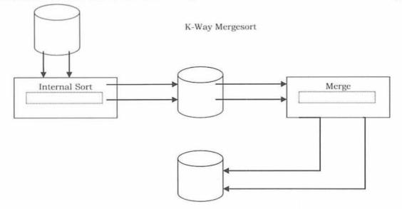
The above algorithm can be generalized by assuming that the amount of data to be sorted exceeds the available memory by a factor of *K*. Then, *K* chunks of data need to be sorted and a *K* -way merge has to be completed.
