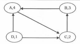
The last step is performing DFS on this reversed graph  $G_r$ . While doing *DFS*, we need to consider the vertex which has the largest DFS number. So, first we start at *A* and with *DFS* we go to *C* and then *B*. At B, we cannot move further. This says that  $\{A, B, C\}$  is a strongly connected component. Now the only remaining element is *D* and we end our second *DFS* at *D*. So the connected components are:  $\{A, B, C\}$  and  $\{D\}$ .
