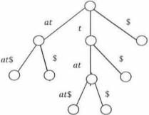
Since there are no more elements, this is the completion of the construction of the suffix tree for string T = tatat. The time-complexity of the construction of a suffix tree using the above algorithm is  $O(n^2)$  where *n* is the length of the input string because there are *n* distinct suffixes. The longest has length *n*, the second longest has length n - 1, and so on.
