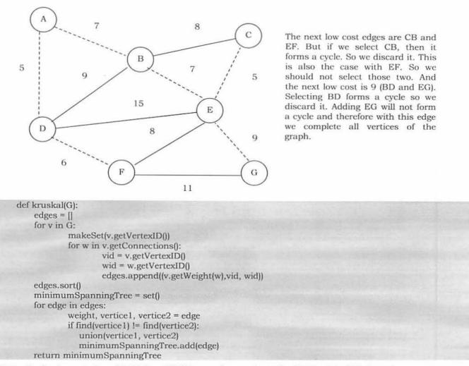
**Note:** For implementation of UNION and FIND operations, refer to the *Disjoint Sets ADT* chapter. The worst-case running time of this algorithm is O(ElogE), which is dominated by the heap operations. That means, since we are constructing the heap with E edges, we need O(ElogE) time to do that.
