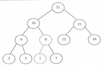
Now the tree is satisfying the heap property. In the above heapifying process, since we are moving from top to bottom, this process is sometimes called *percolate down*. Similarly, if we start heapifying from any other node to root, we can that process *percolate up* as move from bottom to top.
