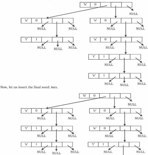
Based on these examples, we can write the insertion algorithm as below. We will combine the insertion operation of BST and tries.
