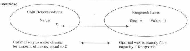
This problem is identical to the Integer Knapsack problem. In our problem, we have coin denominations, each of value  $v_i$ . We can construct an instance of a Knapsack problem for each item that has a size  $s_i$ , which is equal to the value of  $v_i$  coin denomination. In the Knapsack we can give the value of every item as -1.
