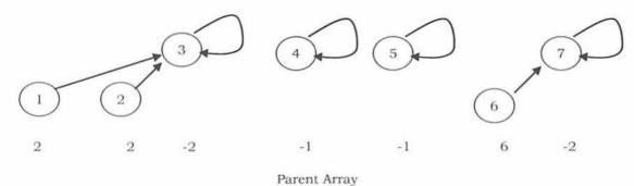
As in UNION by size, in this method we store negative of height of the tree (that means, if the height of the tree is 3 then we store -3 in the parent array for the root element). We assume the height of a tree with one element set is 1. For the previous example (after UNION(0,2)), the new representation will look like:
