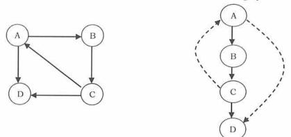
Now, as per the algorithm, performing DFS on this G graph gives the following diagram. The dotted line from C to A indicates a back edge.
