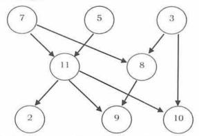
Initially, *indegree* is computed for all vertices, starting with the vertices which are having indegree 0. That means consider the vertices which do not have any prerequisite. To keep track of vertices with indegree zero we can use a queue.
