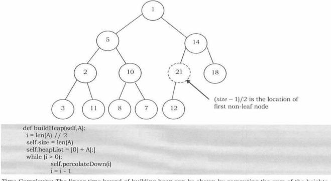
Time Complexity: The linear time bound of building heap can be shown by computing the sum of the heights of all the nodes. For a complete binary tree of height *h* containing  $n = 2^{h+1} - 1$  nodes, the sum of the heights of the nodes is n - h - 1 = n - logn - 1 (for proof refer to *Problems Section*). That means, building the heap operation can be done in linear time (O(*n*)) by applying a *PercolateDown* function to the nodes in reverse level order.
