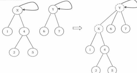
• FIND(X): Returns the name of the set containing the element X. We keep on searching for X's set name until we come to the root of the tree.
