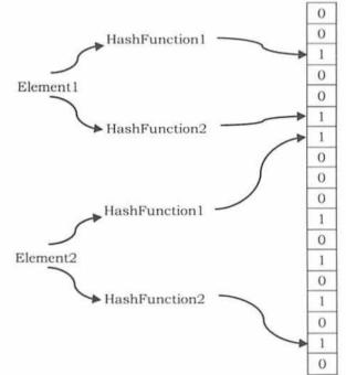
Now that the bits in the bit vector have been set for *Element1* and *Element2*; we can query the bloom filter to tell us if something has been seen before.
