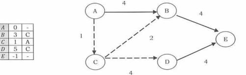
Shortest path to B, D using C as intermediate vertex
