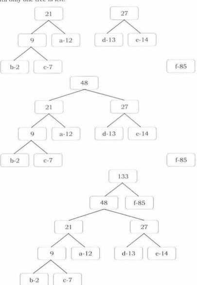
Once the tree is built, each leaf node corresponds to a letter with a code. To determine the code for a particular node, traverse from the root to the leaf node. For each move to the left, append a 0 to the code, and for each move to the right, append a 1. As a result, for the above generated tree, we get the following codes:
