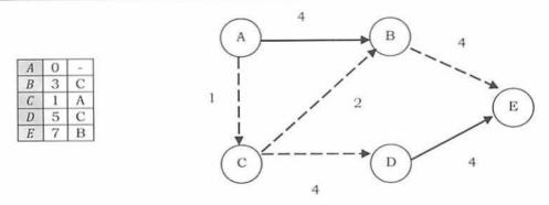
The final minimum cost tree which Dijkstra's algorithm generates is:
