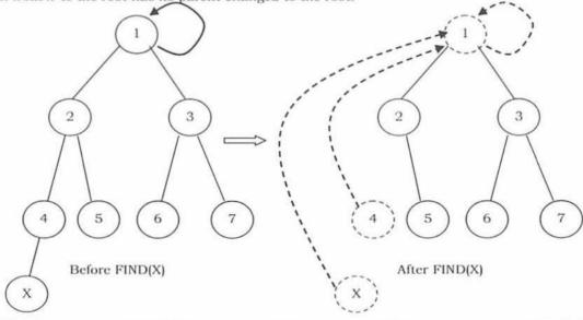
With path compression the only change to the FIND function is that S[X] is made equal to the value returned by FIND. That means, after the root of the set is found recursively, X is made to point directly to it. This happen recursively to every node on the path to the root.
