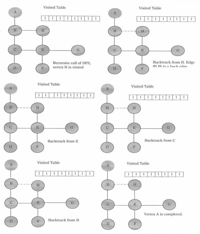
From the above diagrams, it can be seen that the DFS traversal creates a tree (without back edges) and we call such tree a *DFS tree*. The above algorithm works even if the given graph has connected components.
