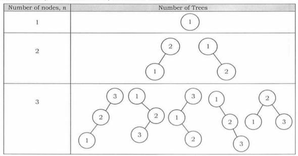
Let us assume that the nodes of the tree are numbered from 1 to n. Among the nodes, we have to select some node as root, and then divide the nodes which are less than root node into left sub tree, and elements greater than root node into right sub tree. Since we have already numbered the vertices, let us assume that the root element we selected is  $i^{th}$  element.
