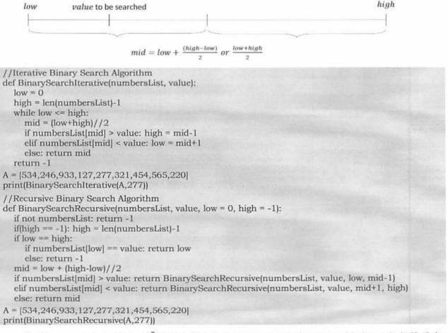
Recurrence for binary search is  $T(n) = T(\frac{n}{2}) + \Theta(1)$ . This is because we are always considering only half of the input list and throwing out the other half. Using *Divide and Conquer* master theorem, we get, T(n) = O(logn).
