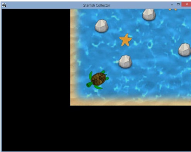
Figure 3-12. Incorrect camera positioning causing the area beyond the game world to be rendered in black
