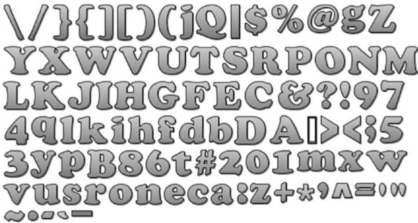
Figure 5-4. An image file (512 by 256 pixels) used to create a bitmap font
