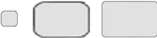
Figure 5-10. A button-like image, scaled using standard methods and using nine-patch methods
