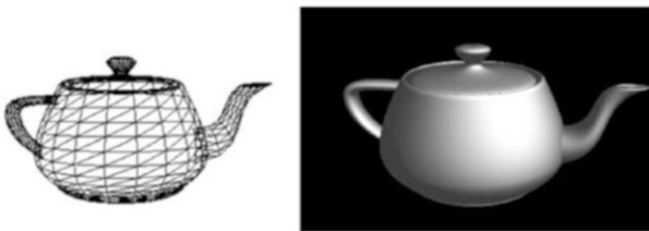
Figure 16-5. The Utah teapot , rendered in wireframe (left) and with material applied (right)
