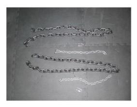
In a matter of minutes you'll be able to assemble the chains and get them ready to go by simply threading one of the smaller 3/16th chains through the last link of one of the thicker chains and then securing the two ends of the small chain in place by attaching a quick link in between! That's it! It's that simple. The two smaller chained loops will now serve as the part that hooks onto the bar and the larger chains will be your variable weights! Here's what your setup will look like now:
