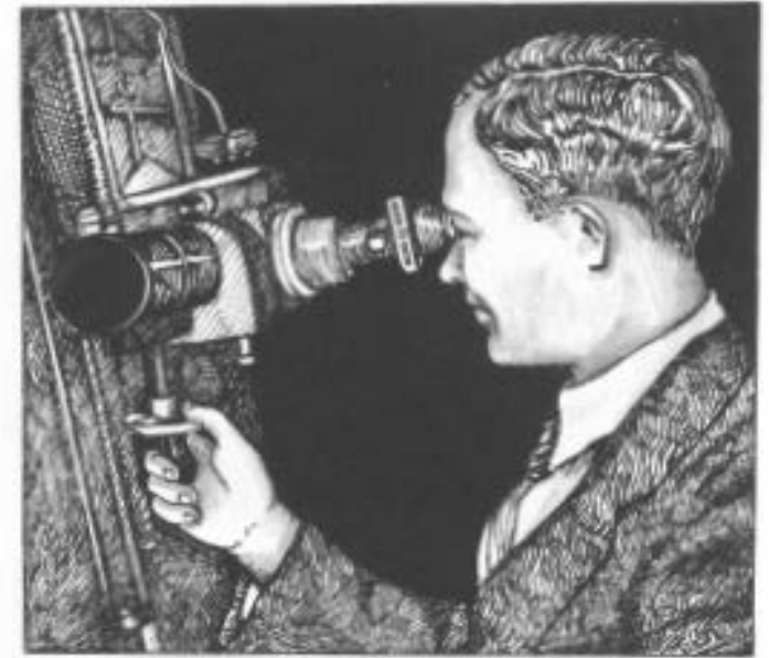
Clyde Tombaugh, the discoverer of Pluto, at the "blink comparator," an instrument used to compare photographs of sections of the sky. Tombaugh found Pluto after comparing the positions of hundreds of thousands of heavenly bodies.
