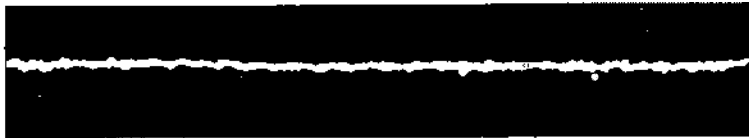
CLOUD CHAMBER TRACK OF A SLOW PROTON
