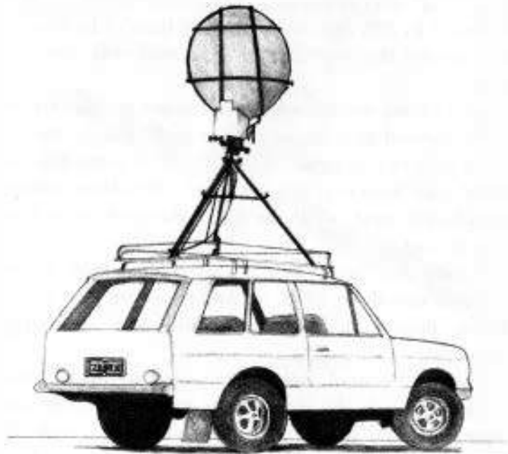
Mobile television unit with microwave antenna
